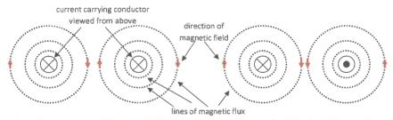
It is the relative direction of the **magnetic fields** and not the direction of current flow which dictates whether the force will be attractive or repulsive. When the currents flow in the same direction, the respective magnetic fields between the conductors are actually opposing each other, therefore fields are unlike and so the force is attractive. The reverse is true when the currents flow in opposite directions, as shown above
